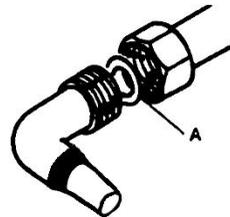
make sure whether the gasket / seal (A) has already installed.
