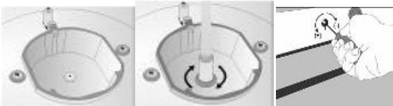
3. Please close nozzle by your finger, open gas valve and check gas leakage by soap form.
