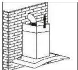
• Sliding the chimney to adjust the chimney height. When the height you required is reached, then hang the fixing hole to the fixing screws as showed in below pictures
