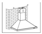
Fix the lower chimney with two pieces of 4x8 mm screws
