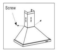
• Sliding the chimney to adjust the chimney height. When the height you required is reached, then fix two pieces of 4x8 mm screws onto the hole fixing with plate I as showed in below pictures
