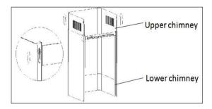
• Drill 2 x 8 mm holes to accommodate the plate II. Screw and tighten the plate II into the wall with two screws provided. Assembly the chimney into the unit and fix it with two screws
