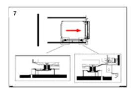
8. Attach the frame microwave from front to relate with the holder.
