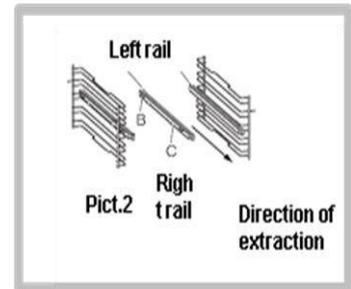
3) Tighten the second frame with guide rails using holes are provided in the wall of the oven. Holes for order lies in the holes left F1, F2 and order on the D1, D2. (see Pict.3).
