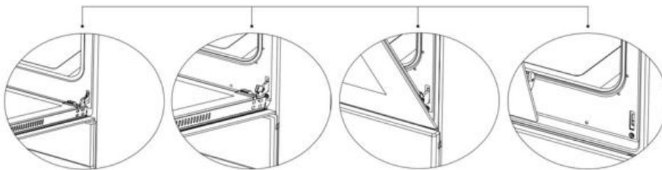
Open the door completely by pulling the oven door toward you. Then, as shown in Figure 7.1, pull the hinge lock up with a screwdriver and perform the unlocking operation.
