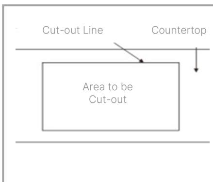
3. Drill the underside of the countertop as shown in the picture below.
