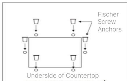
5. Place the fixing brackets over the screw anchors; insert the provided screw, but do not fully tighten it.
