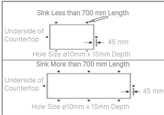
4. Insert the *Fischer* screw anchors into the drilled holes.
