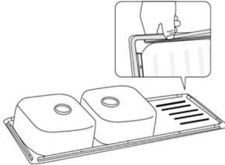
4. Install the anchor bracket vertically underside the sink and pull it up to lock the sink into horizontal position.
