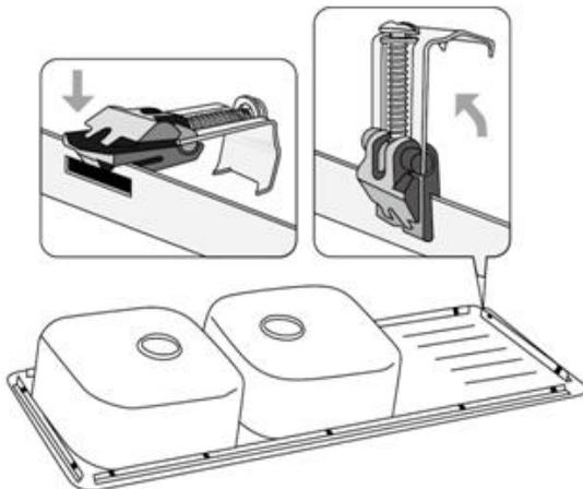
5. These anchor brackets are designed to be used for countertop with thickness 30 - 40 mm (1). If the countertop is thinner, insert the wooden wedges between the countertop and the brackets to secure them (2). After installing two brackets at each corner, install the rest evenly spaced around the perimeter of the sink.
