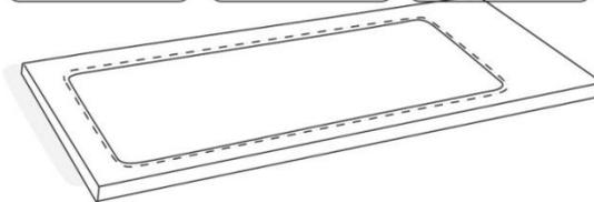
3. Adhere the waterproof seal tape around the underside of the edge of the sink. Lay the sink slowly (without ridges on its seal).
