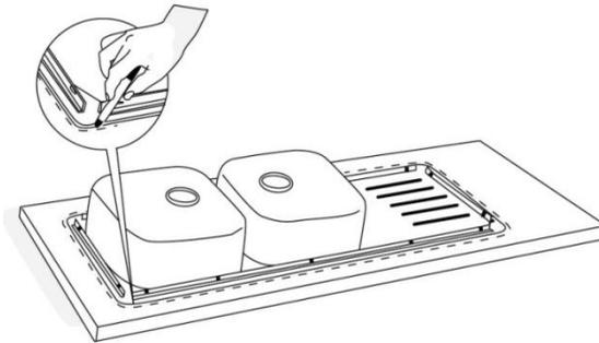
2. Move the sink out of the countertop and draw another line with inner spacing 10 mm (1 cm) from the first line. Drill all four corners with a hole and cut along the countertop following the second line (another option is to use the "cut-out" dimension that provided through the label attached on the product).
