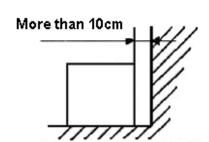
Do not put the freezer near the heat source such as stove, hot plates etc. and avoid placing freezer under direct sunlight which may hamper with the cooling process.
