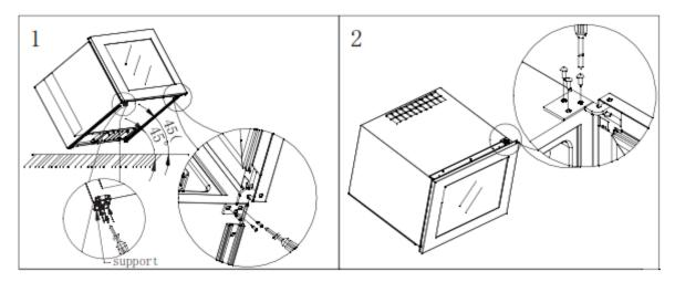
2. Level the wine cooler, hold the door and remove upper right hinge's screws with screwdriver, then take out the door, put the door safety, unscrew 2 screws at the bottom and remove the reed switch, then install at top of frame, and take out the location-plate's screws and fix the location-plate on the other side, and rotate the door 180 degree (Fig.2 & Fig.3 & Fig.4).
