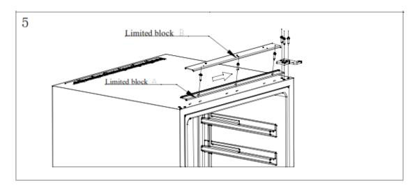
3. Remove the block B following the arrows in picture, then release all the screws on limited block A, and remove the limited block A. Install the limited block A on the right side with screws, then install limited block B, then set the door with screws, then fix the supporter on the bottom right side. (see Fig.5 & Fig.6 & Fig.7).
