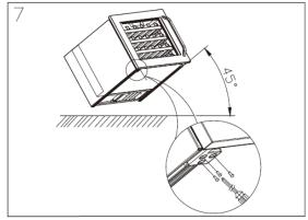
4. Some wine cooler with limited block at the bottom of cabinet. After installing the limited block on the top of cabinet. Then fix the lower limited block with screws according the holes.
