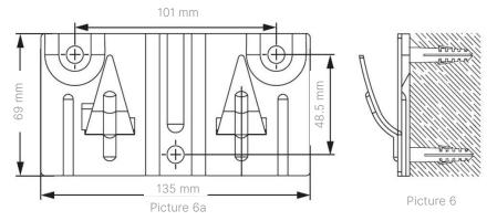
• Methods of installation ES 20SR: after selecting a proper location, determine the positions of the two installation holes that are used for the expansion bolts with the hook (300 mm). Make two holes on the wall with the corresponding depth by using a chopping bit with the size matching the expansion bolts attached with the machine; insert the Fischer screw (M8\*80); tighten the nuts to fix firmly; then, hang this water heater on it (see Picture 6b).
