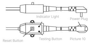
If the indicator lights turn on, the thermostat will automatically control the temperature. When water temperature inside the heater has reached the set point, water heater will switch off automatically. When water temperature falls below the set point, water heater will be turned on automatically to restore the heating.
