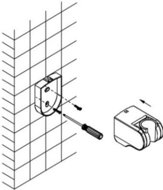
2. Place the rear holder cover; tighten the screws; and install the shower holder.
