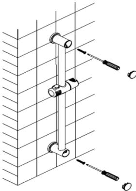
2. Place the sliding bar set into its position. Then, tighten the screws and close the bracket cover.
