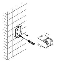
2. Place the rear holder cover; tighten the screws; and install the shower holder.
