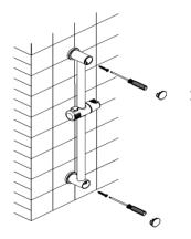
2. Place the sliding bar set into its position. Then, tighten the screws and close the bracket cover.
