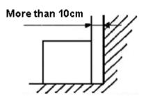
Do not put the showcase cooler near the heat source such as stove, hot plates etc. and avoid placing unit under direct sunlight which may hamper with the cooling process.
