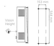
Hang the water heater on the installed bracket and hook bolt by the holes in the backside of the water heater (2 holes in the middle upper part and the other 2 holes in the middle lower of the water heater).
