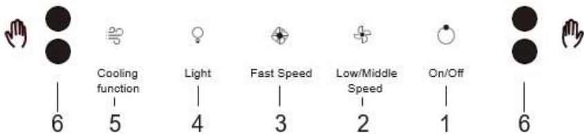
1. On / off key:When this key is touched in the off state,entering the standby state and waiting for other key operations;When you touch this key again, it returns to the off state.Time-delay function:when the motor is running,touch this key to enter a 1-minute time-delay shutdown state,the indicator light flashes during the delay.In the off state,long press this key for 2 seconds to turn off the somatosensory function;long press again for 2 seconds to turn on the somatosensory function.
