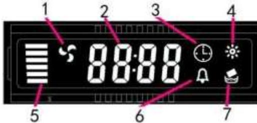
1. Fan symbol will be active when the fan is working
