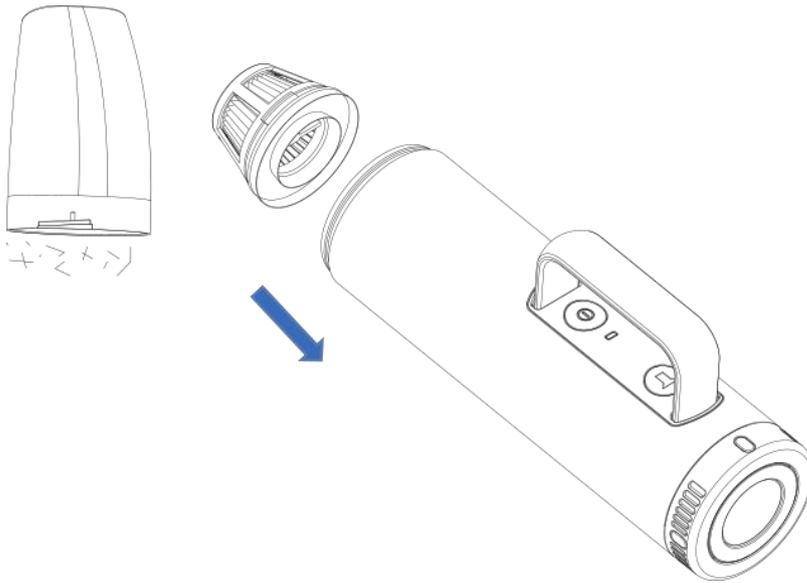
3. Rotate the filter housing clockwise and pull out the filter housing. Take out the inner filter for cleaning or replacement.
