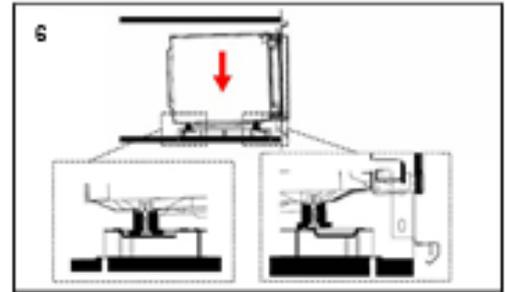
7. To strengthen the position of the microwave, pull forward the microwave until the foot of front side into the hole of buffer / support the front.
