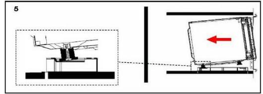
6. Adjust the position of the microwave with the position of the back legs into the holes on the buffer / support the back and most of the front legs into the holes on the buffer / support the front.
