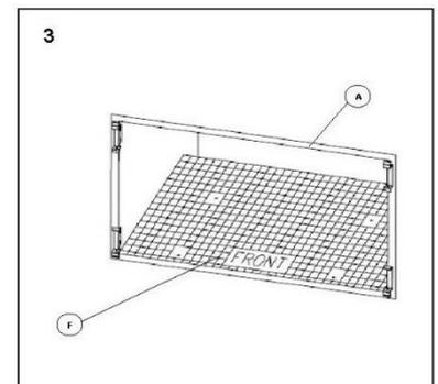
4. Attach both buffer / support with 2 screws on each buffer / support.
