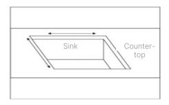
7. Apply sealant to the suitable wet area that recommended for stainless steel sink and countertop material.
