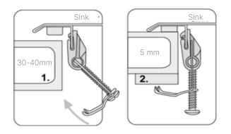
6. Tighten the screws of the anchor brackets to secure the sink in its place.
