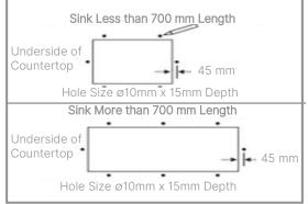
4. Insert the *Fischer* screw anchors into the drilled holes.
