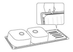
4. Install the anchor bracket vertically underside the sink and pull it up to lock the sink into horizontal position.
