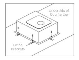
6. Check the alignment between the kitchen sink and the cut-out hole.
