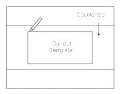
2. Move out the template; cut along the countertop based on the made line using appropriate cutting tool.
