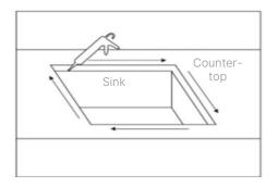
8. Tighten the screws carefully if the sink is already in the desired position, dan remove the leftover sealant around the sink.
