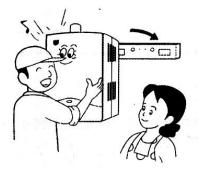
The water heater should be hanged vertically. The standard height of the water heater is adjusted with the parallel position of the flame observation window (peeping hole) to the human eyes.
