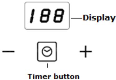
1. "--", default setting. Connect the power, it sounds "Bee" once and display show "--". 5 second later, display turn off automatically.
