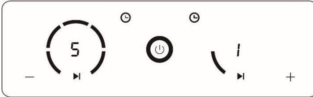
Press ignition button to ignite the flame, the flame will burn in the biggest stage, and LED display will show the number 5.
