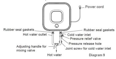
• If the user wants to make a multi-ways supply system, refer to the method shown in figure below for connection of the plumbing.
