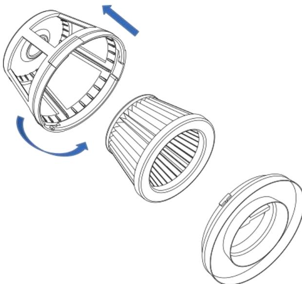
4. Wash the filters under flowing water and let them dry completely
