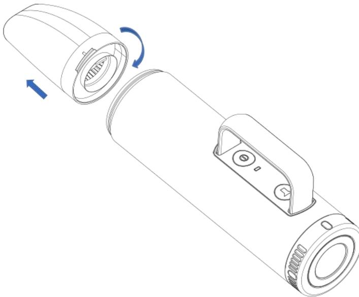
2. Remove the filter housing from the dust cup and clean the dust cup
