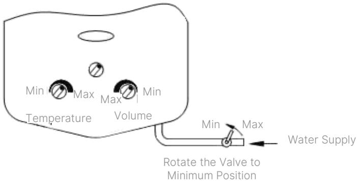
4. Flame can be adjusted by turning the flame controller knob to the 'max' or 'min' position (refer to the illustration picture below).
