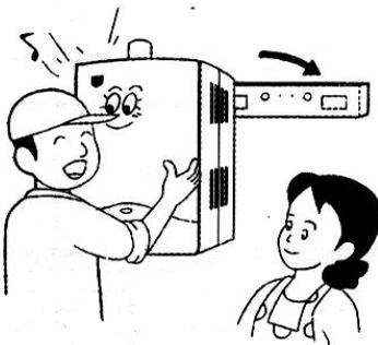
The water heater should be hanged vertically. The standard height of the water heater is adjusted with the parallel position of the flame observation window (peeping hole) to the human eyes.
