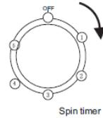
7. After rinsing, put washing materials into the spin tub to spin for 1 to 3 minutes.
