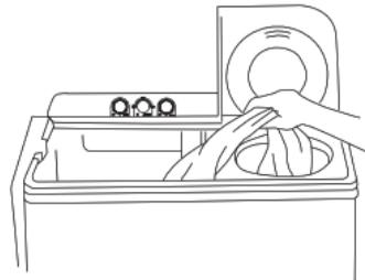
2. To save time, water, and energy, please do the spinning work before rinsing. After spinning, put the clothes into the washtub.
